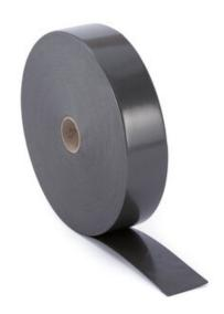
Overlapping auto adhesive band Impactodan is composed of cross-linked polyethylene foam, 3 mm thick and 70 mm wide. It is used as auxiliary product when installing Impactodan's solution for decks. It ensures a correct overlapping between Impactodan rolls, avoiding acoustic short-circuits that could reduce insulation effectiveness.
