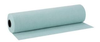
DANOFELT® PP is a non-woven geotextile formed by polypropylene threads, interwoven by needling, without the need or application of chemical binders. It has excellent mechanical and hydraulic behavior. Nonwoven polypropylene geotextiles are used primarily for separation, filtration, and drainage applications. They are typically installed between different layers of soil or other materials to prevent them from mixing together and to improve drainage.
