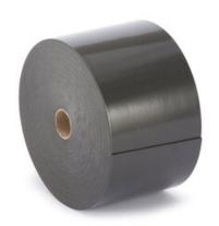
Peripheral band is composed of closed cell cross-linked polyethylene , 3 mm thick and 200 mm wide. It is used as auxiliary product when installing Impactodan's solution for decks. It allows to disband perimeter walls form the mortar deck, avoiding transmission of vibrations trough walls.
