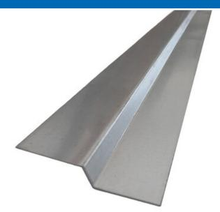
Galvanised sheet metal profiles used to finish off the drainage membrane on vertical surfaces. Prevents the membrane from detaching from the substrate. The fixing of the metal profile to the vertical facing may vary depending on the characteristics of the support.
