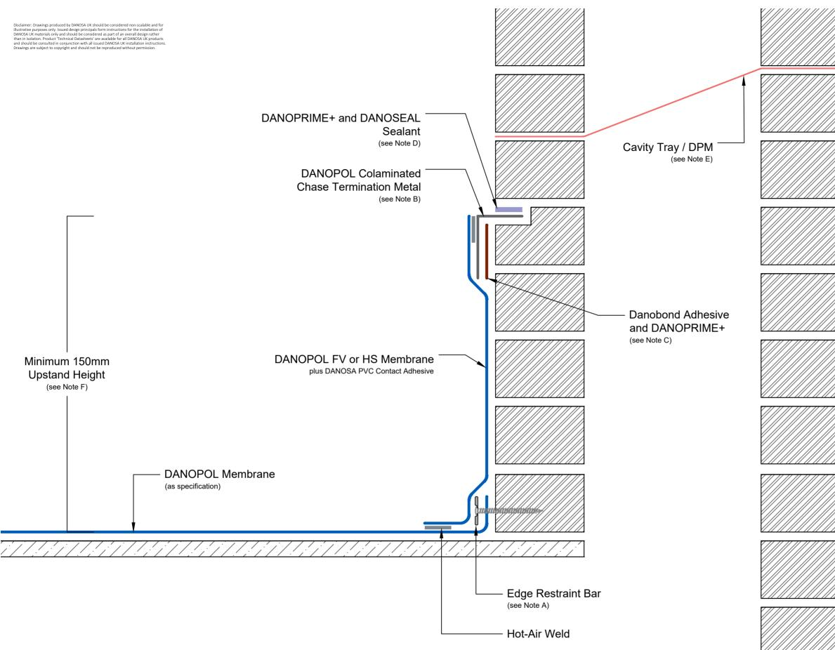
Drawing Number:<br/>DUK-S-(A)-321CRevision:<br/>00Drawing Title:<br/>Abutment with Adhered DANOPOL Metal Chase Flashing<br/>Adhered DANOPOL® Single Ply Membranes - Cold RoofDrawing Number:<br/>00Note of the second second
