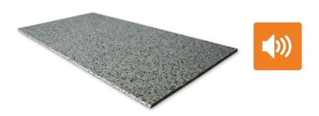
Flexible polyurethane conglomerate panel with high acoustic and thermal insulation properties. ABSORDAN PREN 150 functions acoustically in flooring as an elastic element in a mass-spring-mass system or as an absorber between lightweight elements. It is ideal for renovation and DIY due to its easy installation. In new construction it meets the highest acoustic requirements. Its large format allows for greater surface coverage. Made of 100% recycled materials.
