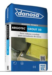
ARGOTEC GROUT 50 is a cementitious mortar (CC), single-component, self-levelling, high-strength and shrinkage-compensated for all types of fillings and anchors, formulated based on a mixture of hydraulic binders, selected aggregates and additives that provide excellent adherence and a great anchoring capacity.
