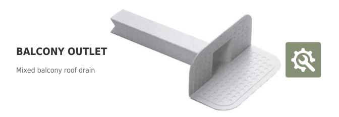
White TPE mixed balcony roof drain with an external cross-section of  $50 \times 45$  mm, compatible with all bitumen membranes by heat welding. Perfectly resistant to flame, corrosion and weathering, it is ductile and easy to handle. Made in one piece, the roof drain has an embossed support base to facilitate bitumen penetration. The hose has a spout at the end to facilitate drainage.
