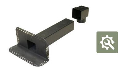
Horizontal outlet EPDM rubber roof drain with an external section of 92 x 92 mm, for downpipe with an outlet diameter of 100 mm. It is made up of two parts: support base-sleeve and connection with vertical downpipe. The cup has an embossed support base to facilitate the penetration of the bitumen. It is compatible with all bituminous membranes by heat welding. Perfectly resistant to flame, corrosion and weathering, it is ductile and easy to handle.
