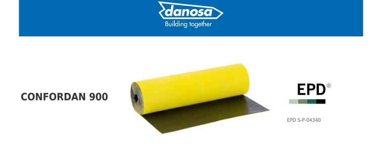
CONFORDAN 900 is a two layer product made of a self-adhesive high density bitumen membrane thermally bonded to a cross-linked polyethylene. CONFORDAN 900 acoustically works as shock absorber in mass-spring-mass system in floor, and removing resonant frequencies in plasterboard system.
