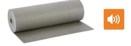
CONFORDAN® ECO is a flexible, chemically cross-linked polyethylene film, closed-cell on one side, which gives the product an elastic internal structure. It's designed to insulate residential wooden floor systems and complements the IMPACTODAN system. Compatible with underfloor heating.
