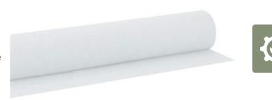
DANECRAN 100 is a 100 g/m² thermo-welded glass fibre felt, used in unbonded solutions as a separating layer between the substrate and the waterproofing membrane. It complies with the specifications required in the UNE 104-204 95 standard.
