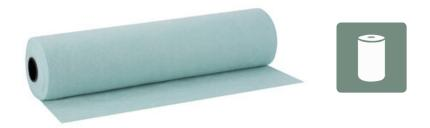
DANOFELT® PP is a non-woven geotextile formed by polypropylene threads, interwoven by needling, without the need or application of chemical binders. It has excellent mechanical and hydraulic behavior. Nonwoven polypropylene geotextiles are used primarily for separation, filtration, and drainage applications. They are typically installed between different layers of soil or other materials to prevent them from mixing together and to improve drainage.
