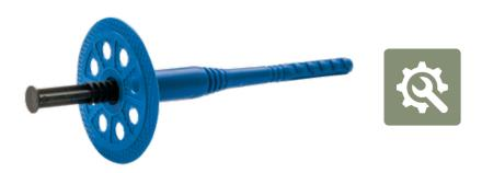
Polypropylene expansion plug with a diameter of 8 mm for fixing insulating panels in the DANOTHERM® SATE external thermal insulation system. With approval ETA06-0242 according to ETAG014 for use category B (solid brick) and C (hollow brick).
