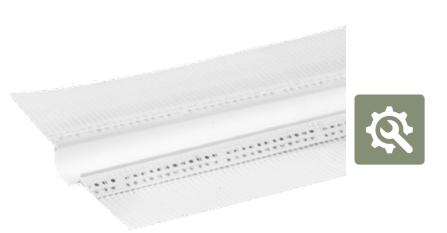
Gasket with heat-welded fibreglass mesh to be installed between the insulating panels in cases of structural joints of the building or where it is necessary to ensure adequate expansion for the absorption of settlement movements in continuous walls.
