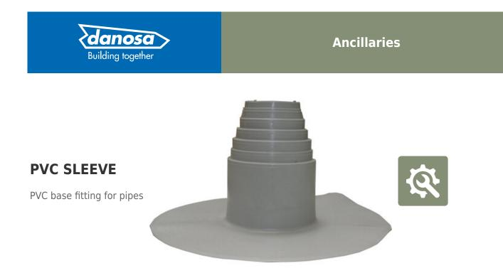
A PVC base fitting for pipes. Compatible with tubes that have a diameter of 75-125 mm. Designed for all DANOPOL membranes.
