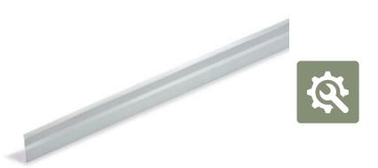
These are galvanised sheet metal profiles used to finish off the waterproofing on parapets and vertical faces, thus preventing the sheet from detaching from the substrate. They are finished with JUNTODAN E or a silicone bead to prevent water from entering between the substrate and the sheet. The fixing of the metal profile to the vertical wall may vary depending on the characteristics of the substrate.
