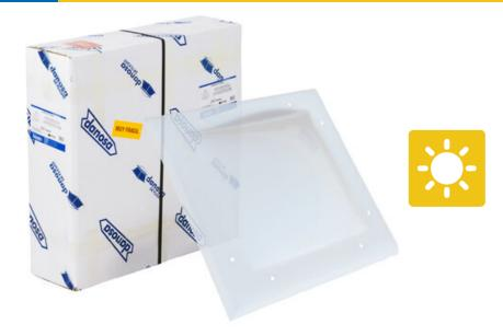
Upper element that is installed under the dome to create an intermediate chamber and prevent condensation. It is manufactured by thermoforming from a 3 mm thick methacrylate sheet.
