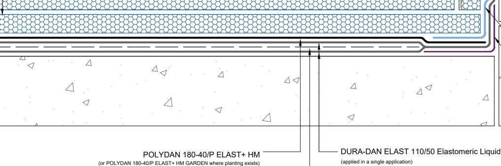
**DURA-DAN REINFORCEMENT MESH** (embedded in DURA-DAN ELAST 110/50 elastomeric liquid)
