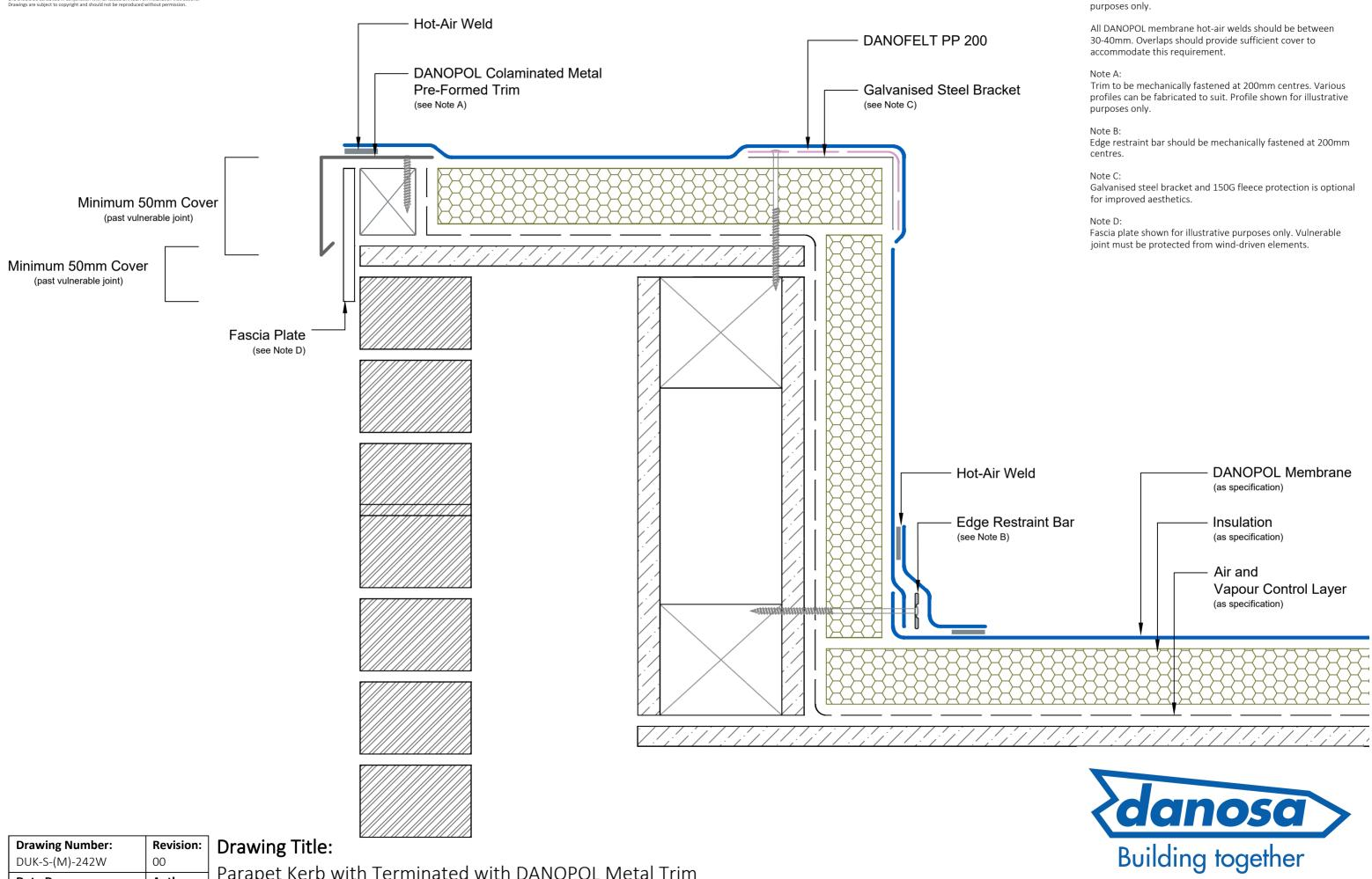
Parapet Kerb with Terminated with DANOPOL Metal Trim Mechanically Fastened DANOPOL® Single Ply Membranes - Warm Roof
