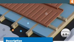
Rehabilitation of single-family homes with wooden structures, leaving the wood exposed. Compatible with installations on the floor. Compression resistance.
